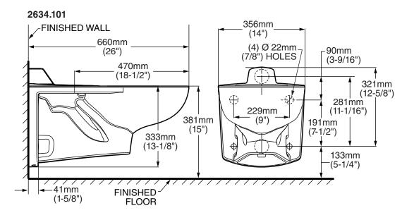
● Toilet designed to meet ADA accessibility standards when top of seat height set at 432 to 483mm (17" to 19") from finished floor.
